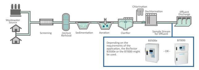
For a wastewater treatment plant effluent water monitoring, a single-stream BioTector TOC analyzer can be used to monitor the quality of the effluent stream to ensure it is ready to be discharged.
