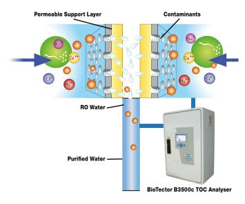
For water treatment applications using a reverse osmosis system, Hach's BioTector B3500c TOC analyser monitors total organic carbons in the purified water stream, to ensure the RO system is performing at the highest level of efficiency.
